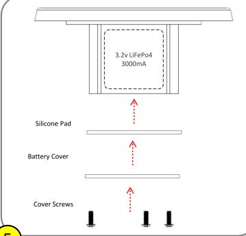
Use the provided wrench and screws to secure the silicone pad and battery cover. Fully tighten screws to ensure the chamber is waterproof.
