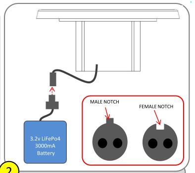
Connect Battery: Caution! When plugging battery connectors together, align notches before joining both connectors. Forcing or connecting backwards will damage the light.
