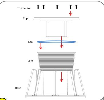
6 Use Provided wrench and top screws to assembly your light together. NOTE: The seal must be in the correct position before tightening down the top to the base.
