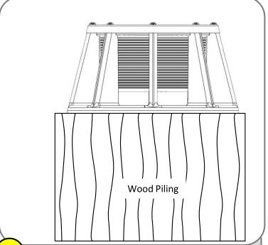
Verify that the top screws are tight to provide a good seal for the lens. Verify that the base of the light is secured to the piling.
